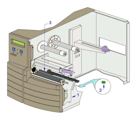
Figure 6-7, Label Sensor Positioning
